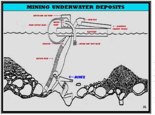
To left is a simplified drawing of a typical suction dredge operation. In most cases, the goal is to reach and clean the underlining bedrock
