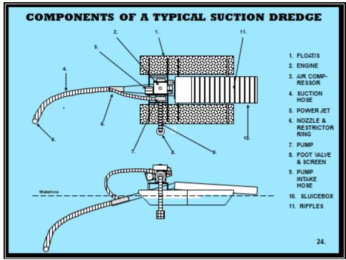
Suction dredges are highly portable. Most can be disassembled and easily packed into areas and reassembled, allowing miners to work virtually anywhere to depths of 20 feet or more without diverting the streams
